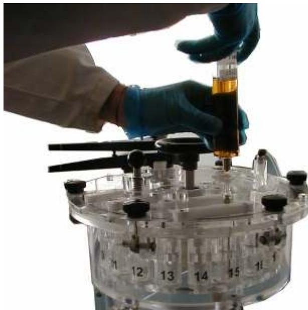
8. Positioning the plug on the vial:
